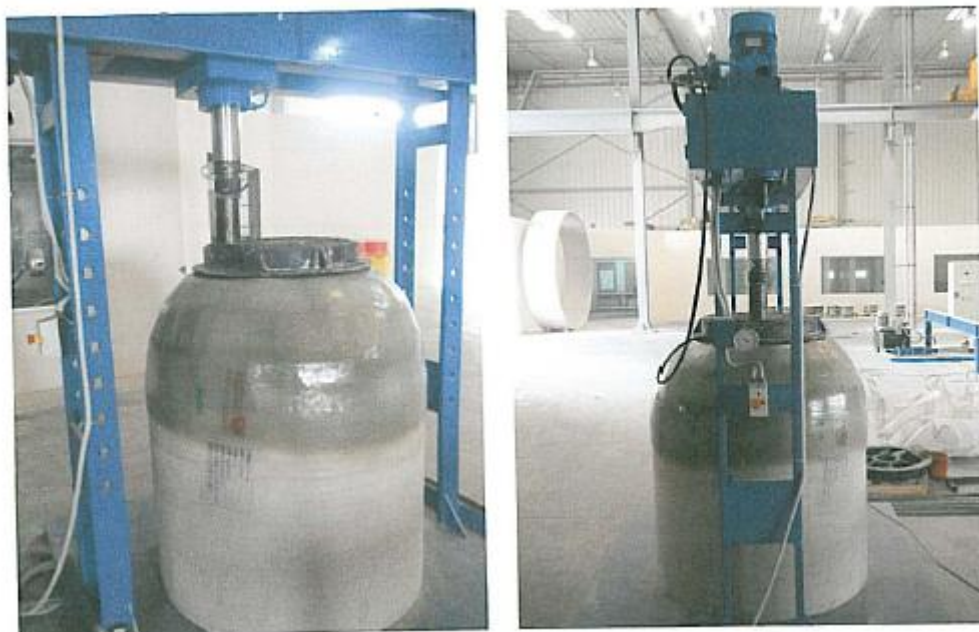
Figure 6: Sample Manhole Test conducted at Tamdid Pipes
