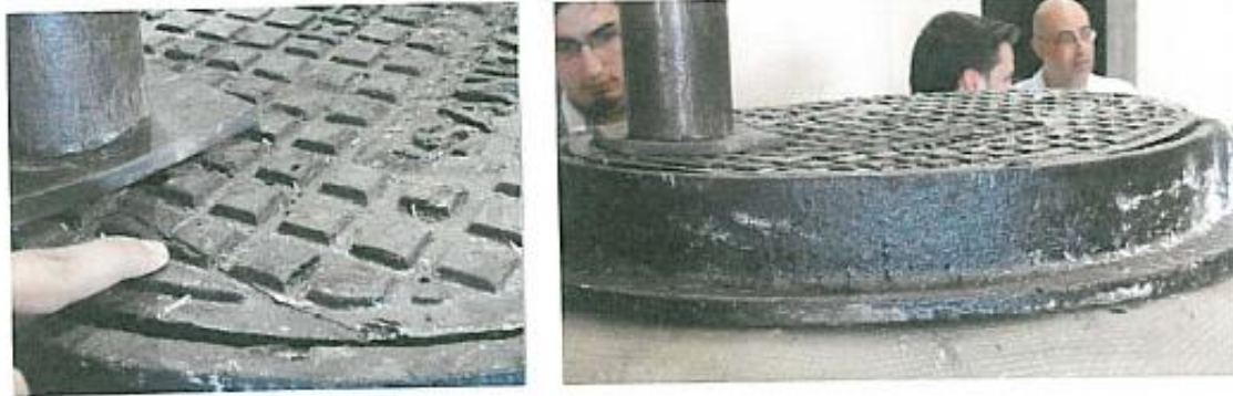
Figure 7: Load Plate Damage
