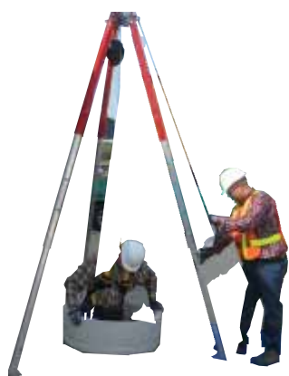
PRO-4 Rescue Tripod shown being used as standard Tripod setup
